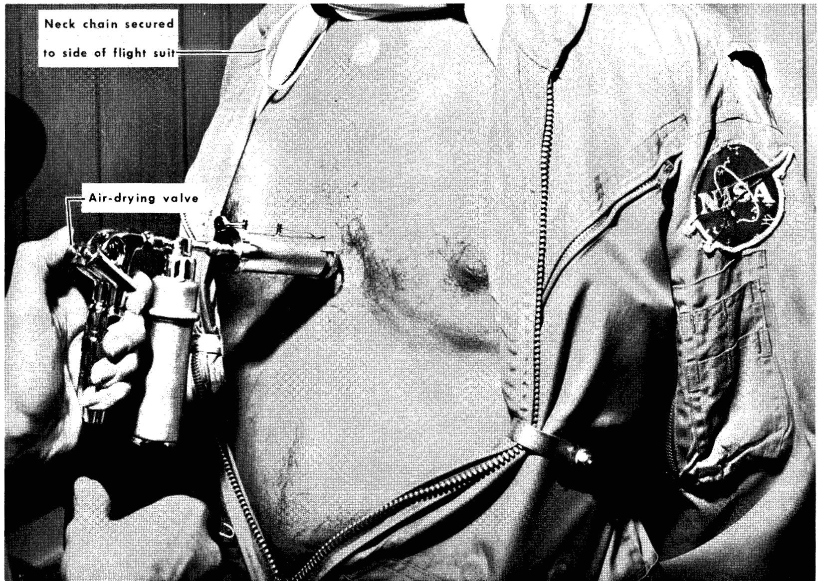
Figure 12.- Spray gun moved back 1/2 inch while air-drying electrode.
