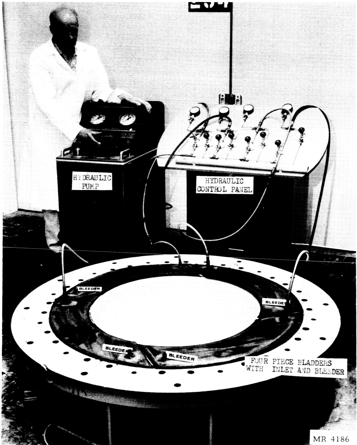
HYDRAULIC SYSTEM AND SECTIONAL BLADDERS FOR FLANGE CONTROL SHOWN ON 28" PLASTIC DIE
