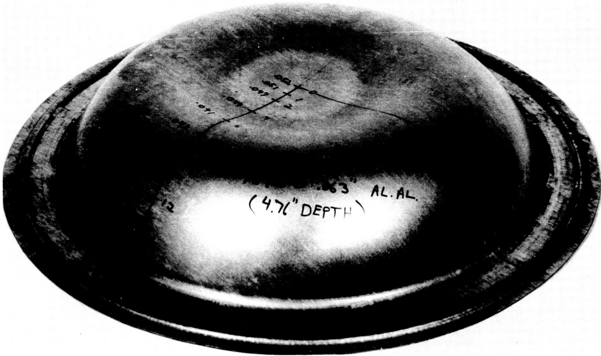
SHAPE OF SPECIMEN 14 AFTER 6 STRETCH FORMING DISCHARGES AGAINST AN INVERTED PUNCH
