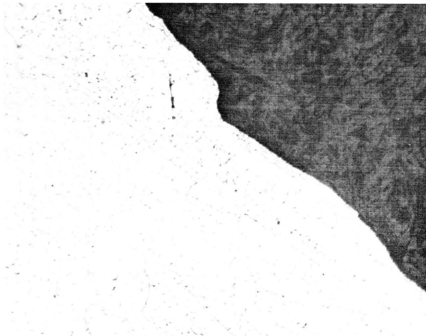
FIGURE 13 - Weld Fracture of the 2400°F Transverse D-43 Weld Tensile Specimen
