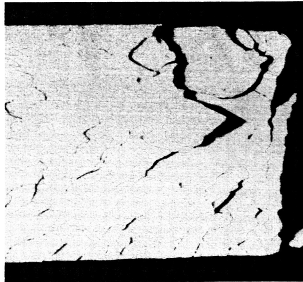
11,730F 80X Weld Specimen, Weld Fracture
