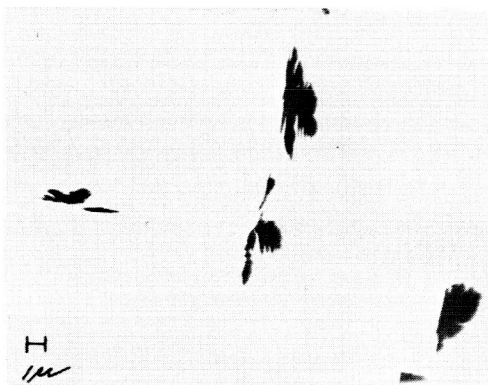
(b) Extraction Replica-Platelets 2500X
