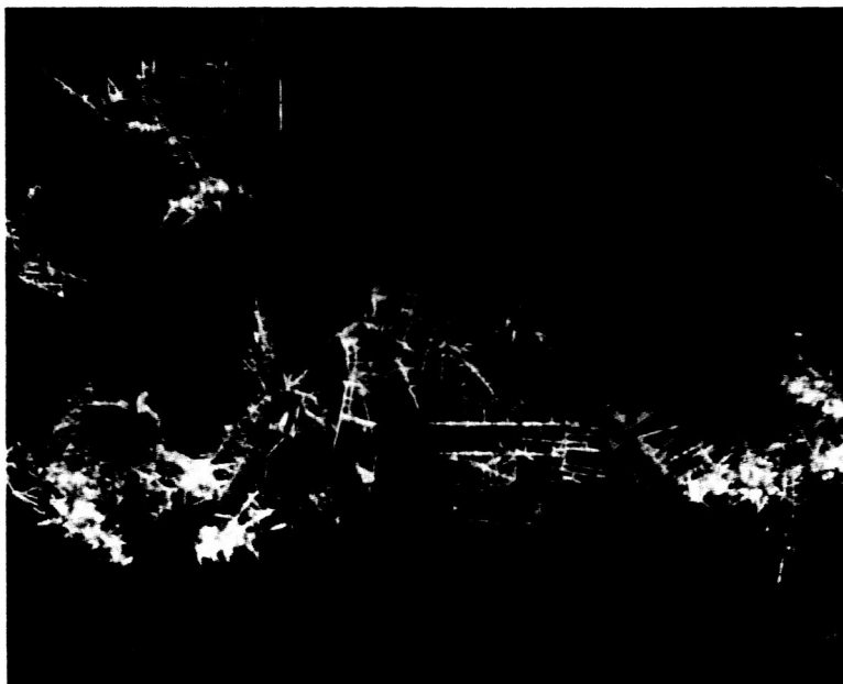
Figure 7b. Non-Adherent Portion of the Deposit Obtained After 27 \text{ C/cm}^2 , 15 \text{ mA/cm}^2 , from 43% KOH, 1.13 M Zn (II), 30^\circ \text{C} , Plus 4.6 g/l Pb (II) as Nitrate. Magnification: 150X
