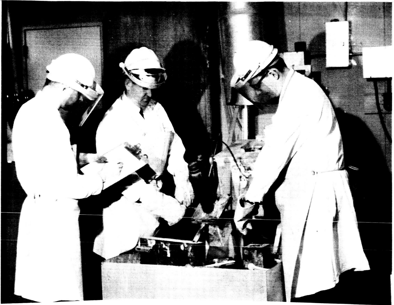
Figure 6. Melting and Casting of Magnesium Alloys At the AMF Research Foundry. The Metal is being poured directly into the Sprue of a cast iron permanent mold. The Crucible is tightly sealed and purified argon protects the liquid metal from oxidation.
