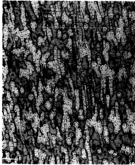
Alloy II-4, Modified, As Rolled, 1\frac{1}{2} Th, 0 Cd, 50 Minutes at Temperature Tensile Strength 38,800 psi Elongation 17.3% 75X
