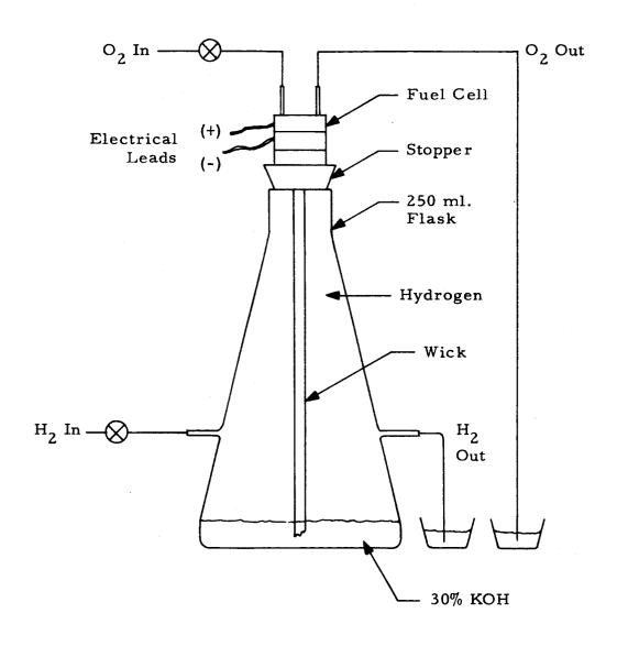
Figure 8. Schematic Diagram of Dead End Flow Tests with Wicks
