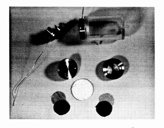
Figure 6. Modified Miniature Fuel Cell
