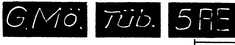
Fig. 3: MINIATURIZED LETTERS (of less than 1 micron) ENGRAVED ON THIN COLLODION FILM USING ELECTRON MICROBEAM PROBES PRODUCED BY DEMAGNIFICATION IN AN ELECTRON MICROSCOPE. (G. Mollenstedt and R. Speidel, Physik. Bl. 16 , 192, 1960)
