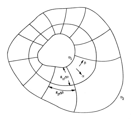
Fig. 1 Schematic of Arbitrary Bearing Surface Described in Curvilinear Coordinates
