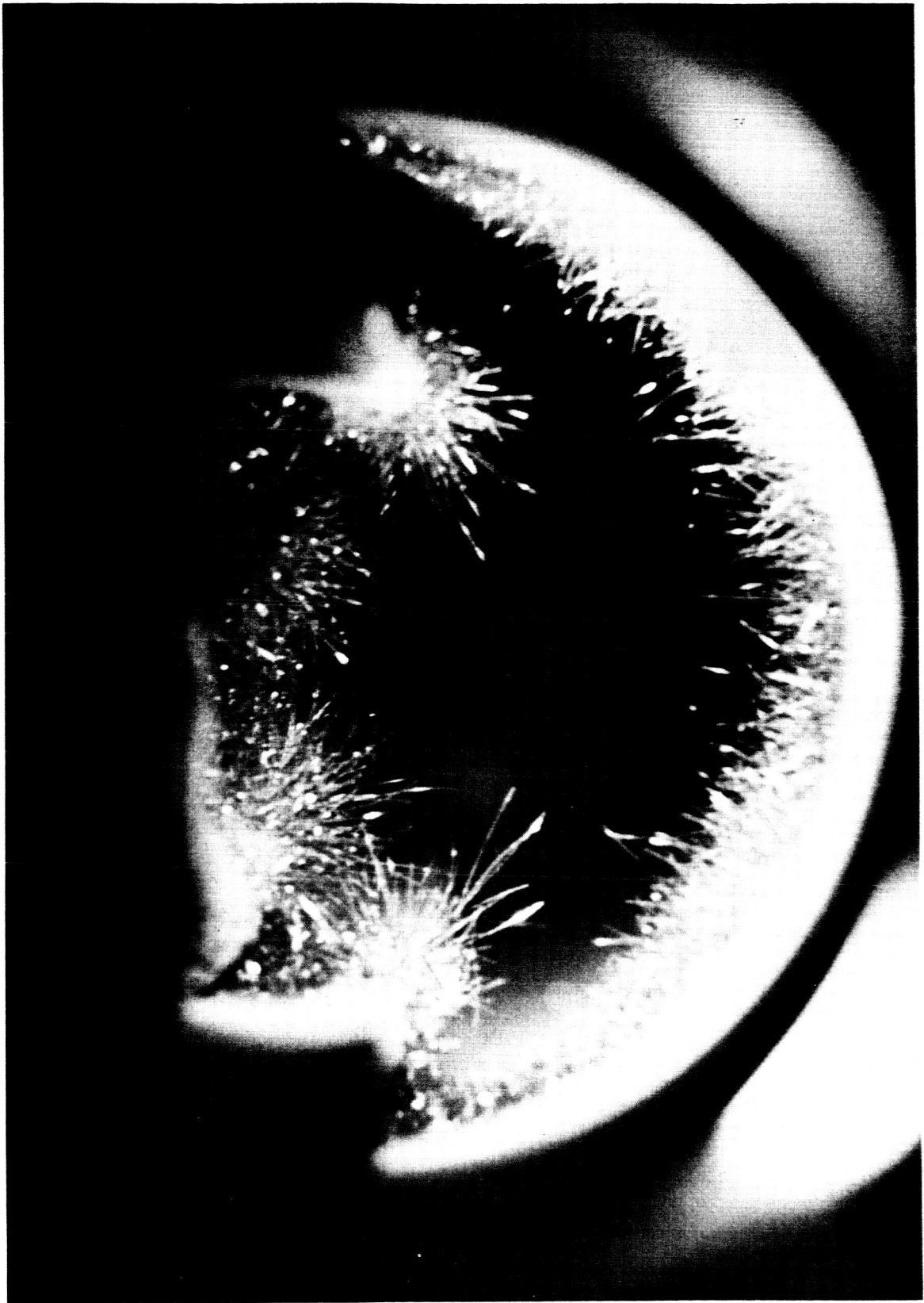
Figure 4. Photo at 6X of Whiskers Grown at End Sections of Radial Furnace
