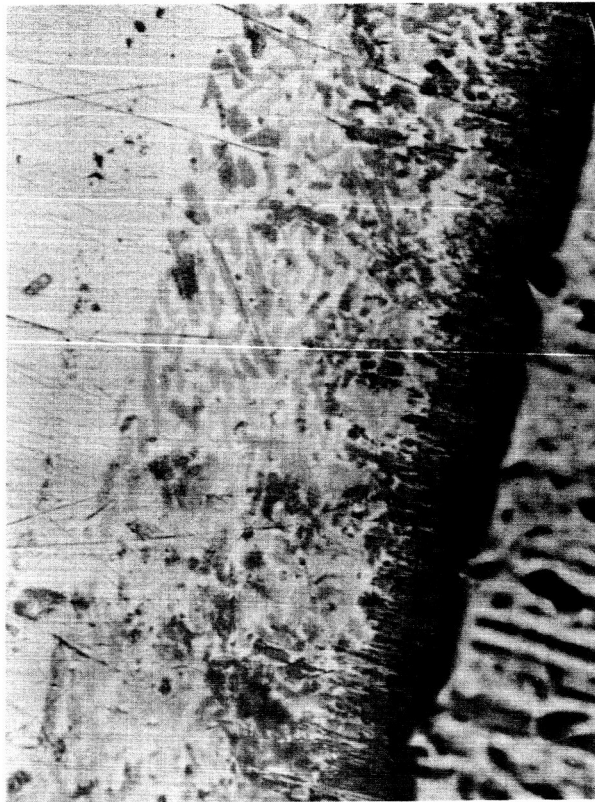
Fig. 6a Precipitation in SnTe braze layer on Ta electrode (top right). X 500
