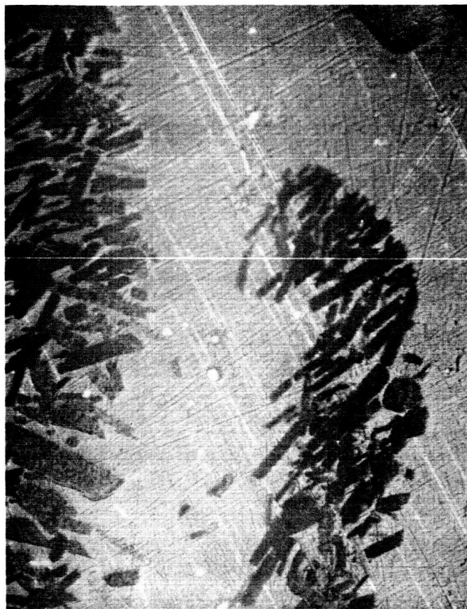
Fig. 2 Alloy A-1-Ta (see text) PbTe and Ta held at 965°C for 20 hours. X 200
