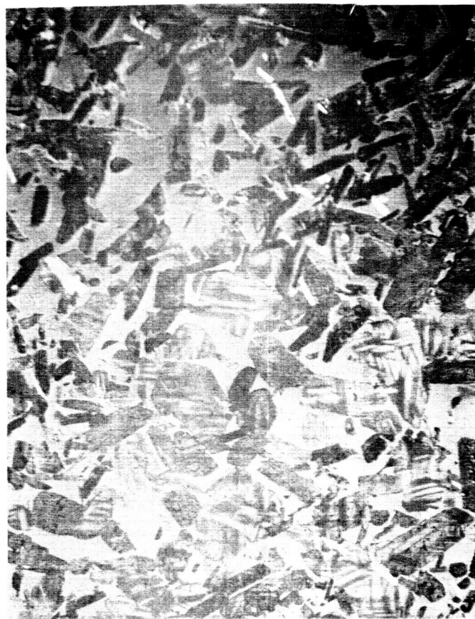
Fig. 2 Alloy A-1-Ta (see text) PbTe and Ta held at 965°C for 20 hours. X 200
