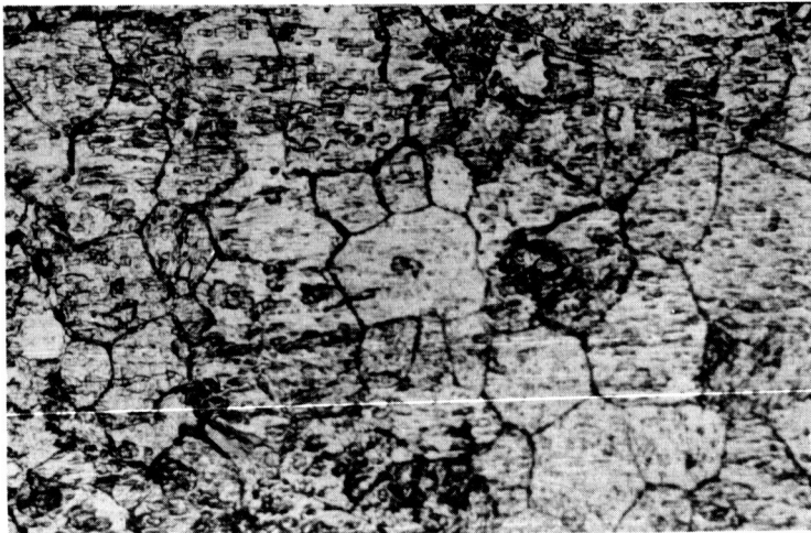
FIGURE 14 (CONT.) TYPICAL MICROSTRUCTURES. (D) (E) AND (F): LONGITUDINAL SECTIONS OF BILLETS M2N-1-2 (MgO-3), M-1-4 (MgO-4), AND M-1-12 (MgO-5) RESPECTIVELY
