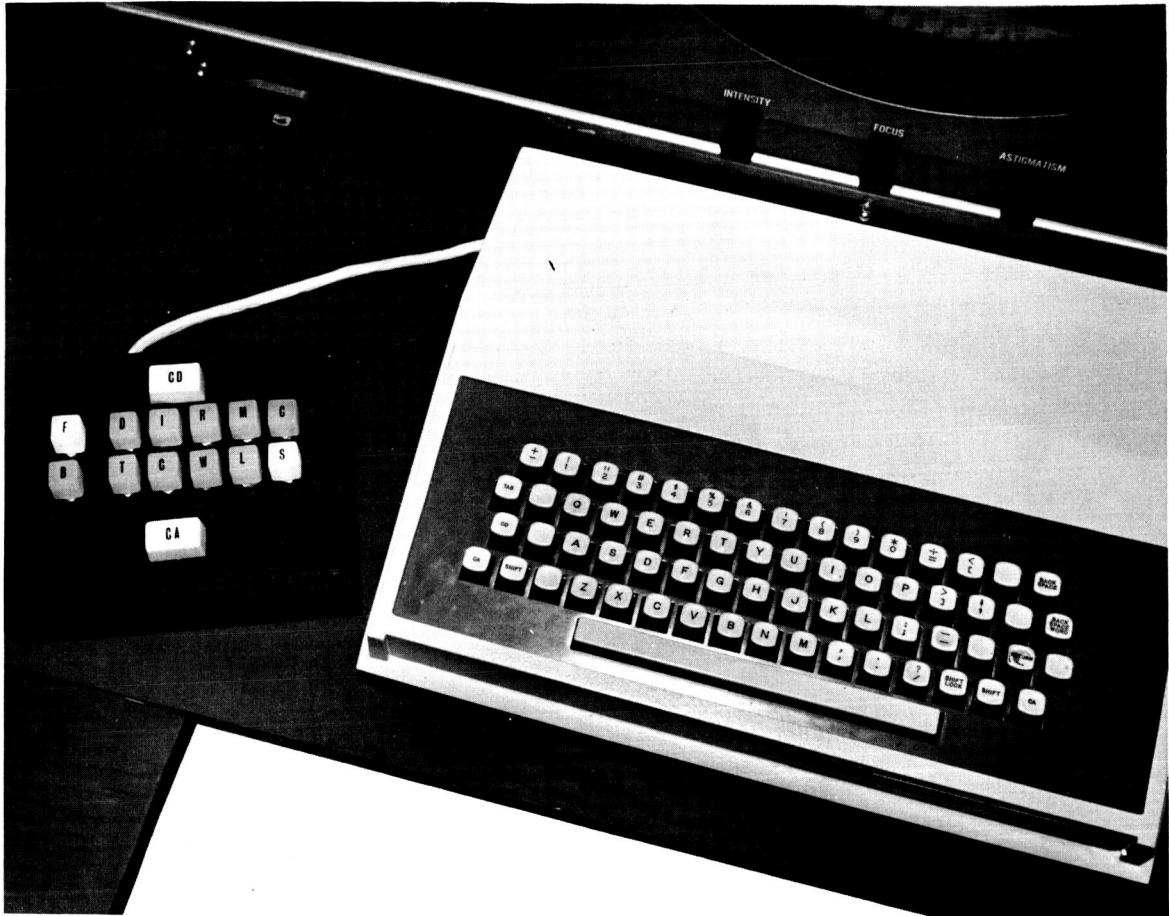
FIG. 17 PUSH-BUTTON PANEL (With Forward Statement Operator Indicated by Push-Button Lights) AND ON-LINE KEYBOARD
