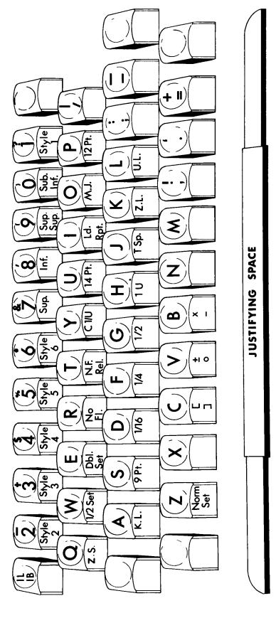
Note that control signals and special characters available only in Control Shift condition are engraved on the vertical faces of the keys.
