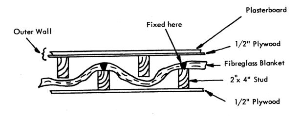
Figure 1b. Recommended Construction
