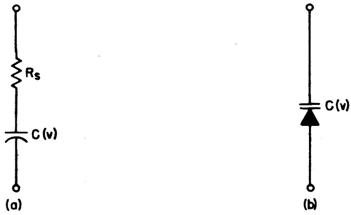
FIGURE 2 (a) THE APPROXIMATE EQUIVALENT CIRCUIT OF A VARACTOR DIODE (b) THE SCHEMATIC REPRESENTATION OF A VARACTOR DIODE
