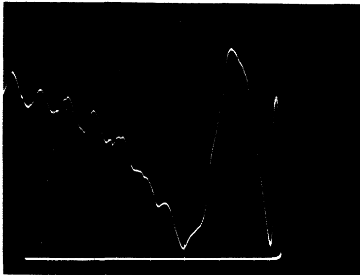
FIGURE 14 ISOLATION CHARACTERISTICS FOR MODE ONE SWITCHING
