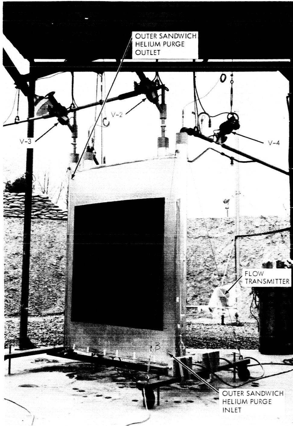
Figure 70. Close-Up of LH 2 Tank and Control Valves
