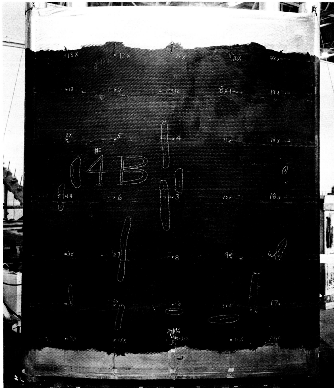
Figure 85. Panel B of LH 2 Tank No. 4 after Test, Showing Cracks in Outer Skin
