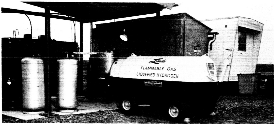
Figure 44. Calorimeter Test Setup - LH 2 Supply Tank
