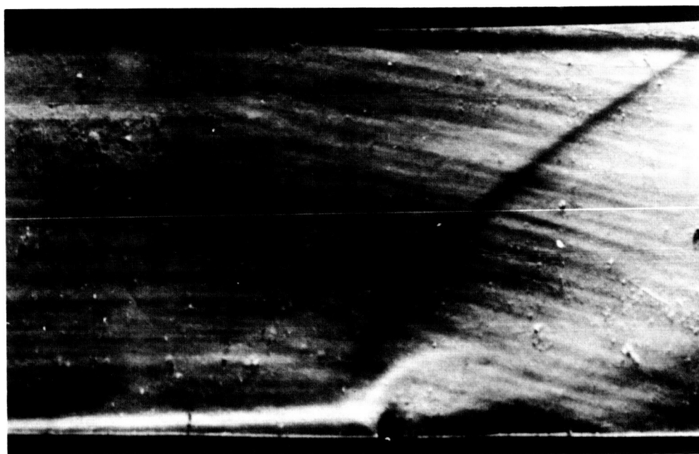
Fig. 3d. Schlieren photograph, nozzle wall; M_\infty = 2.56 , Re = 1.3 \times 10^5 per in.; laminar boundary layer
