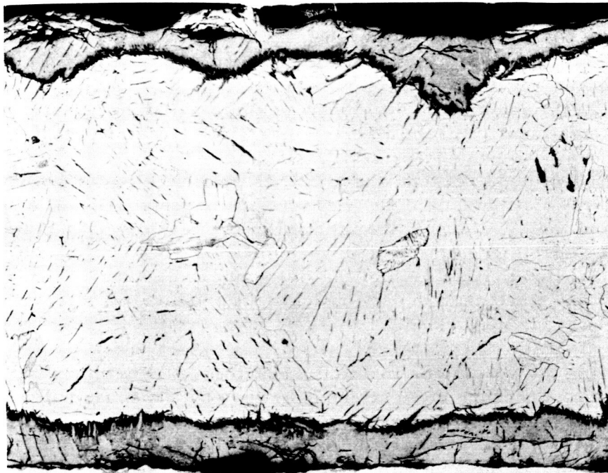
FIGURE 2. Ti-50A SLOW COOLED FROM ABOVE BETA TRANSUS, AFTER 10-HOUR EXPOSURE TO HYDROGEN AT 300 F AND 315 PSIA
