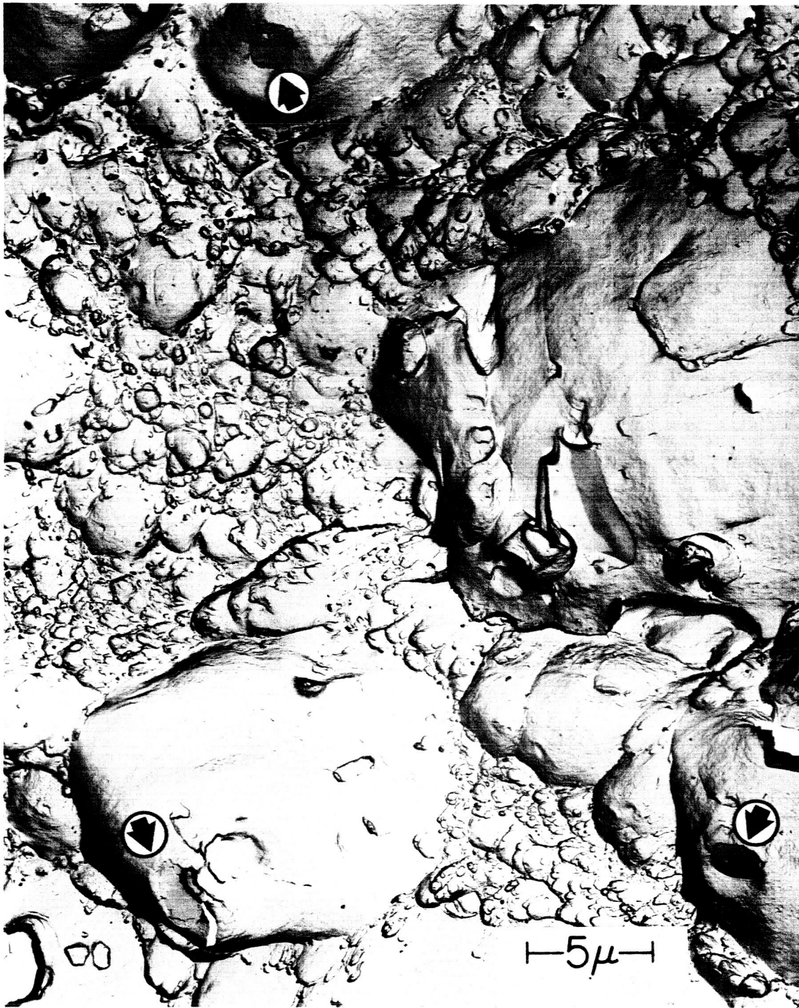
FIGURE 15. FRACTURE SURFACE OF 2219-T87 BASE METAL TENSILE SPECIMEN. (Fractograph taken in central "fibrous" region. Note the range of size of dimples. Arrows indicate origin of larger dimples at second-phase platelets.)
