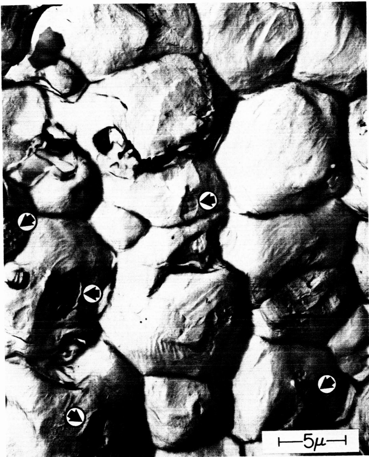
FIGURE 17. FRACTURE SURFACE OF 2219-T87 WELDED JOINT TENSILE SPECIMEN. (Specimen tested with weld crowns machined off. Fractograph taken from location near root of weld passes. Note the large, uniform equiaxed dimples. Arrows indicate origin of voids at second-phase platelets.)
