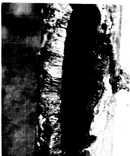
FRONT VIEW, CLOSE-UP OF RUPTURE CENTER SECTION.
