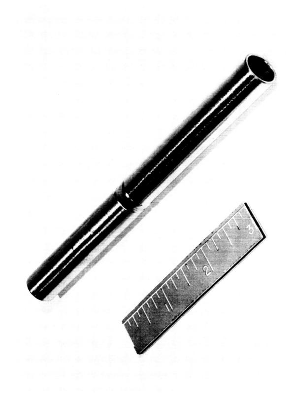
FIGURE 2. Weld Between Cb-1Zr Crucible and Mo-2Ti Collector Tube (View Showing Open End of Collector).
