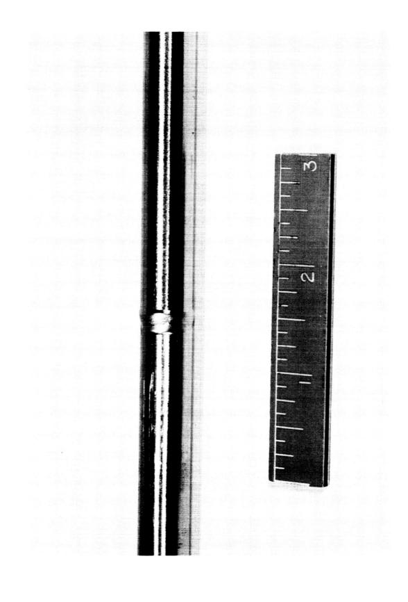
FIGURE 1. Weld Between Cb-1Zr Crucible and Mo-2Ti Collector Tube (View Normal to Axis).
