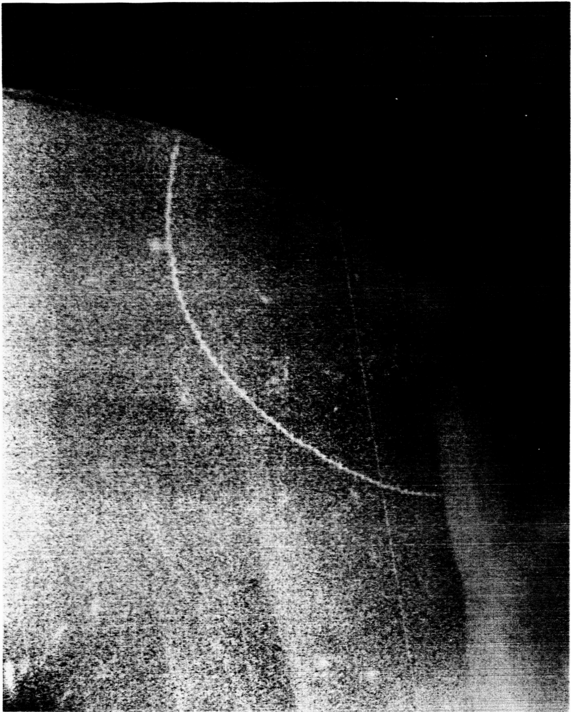
Fig. 7. Enlarged portion of the 56-sec coronal exposure, No. 19, showing the track of a distant sunlit particle. Pointing jitter caused the track to be roughly sinusoidal. The particle was in the field during most of the exposure.
