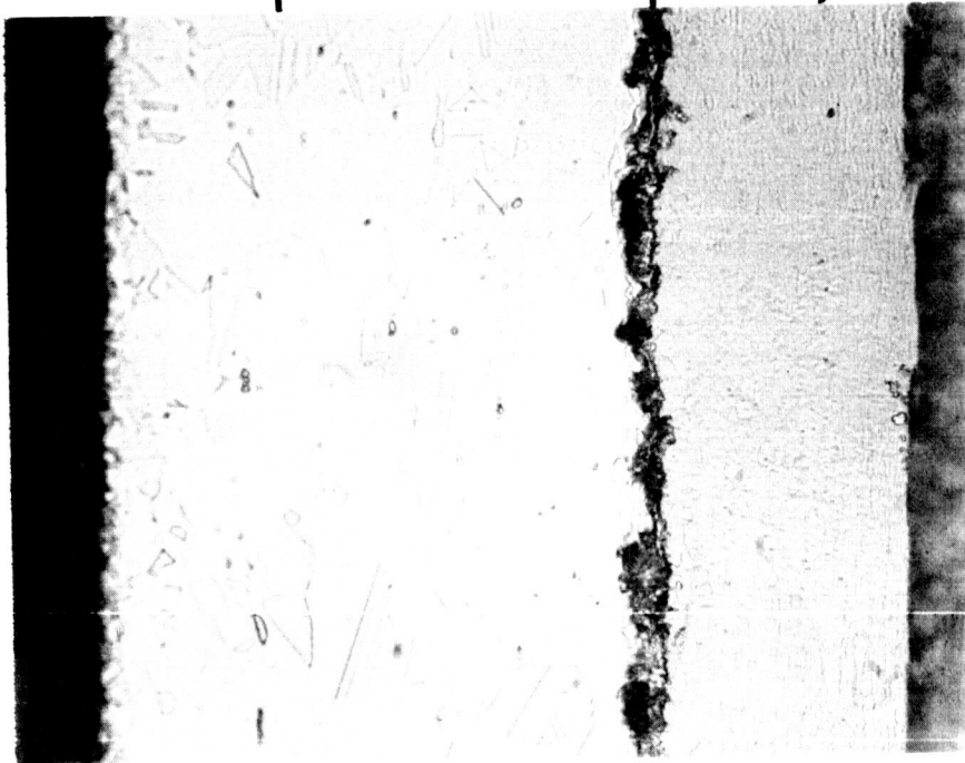
FIGURE II. B-14. Micrograph Showing Suspected Inconel 600-Columbium Reaction Zone in 1600°F Aging Specimen Using Dispersion-Strengthened Copper Core Material.
