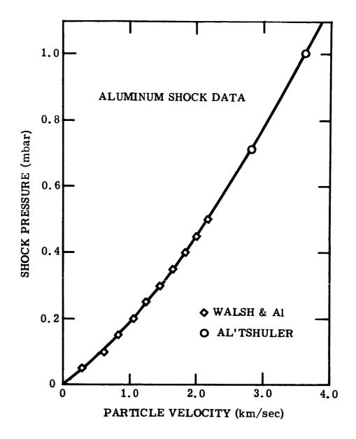
Figure 3 Shock-Wave Pressure vs Particle Velocity in Aluminum
