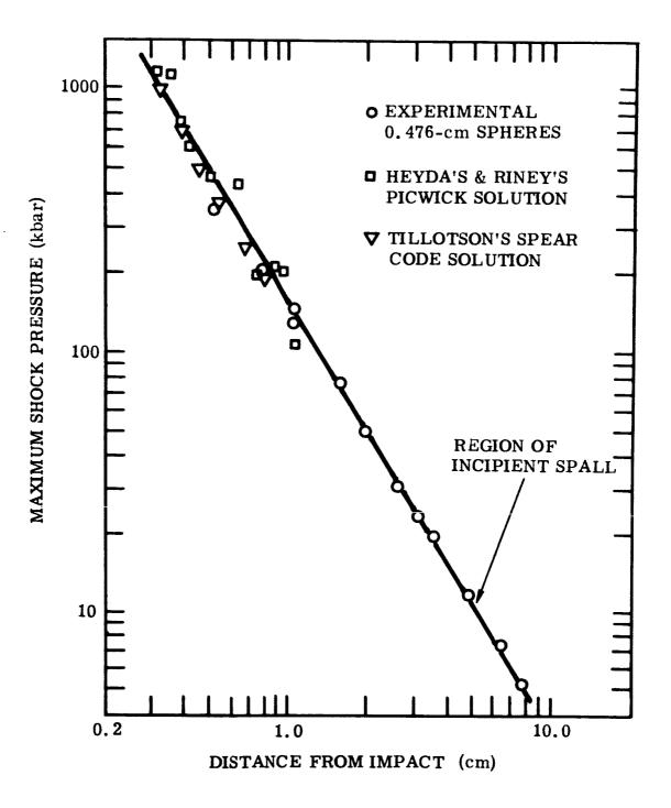
Figure 4 Calculated and Measured Maximum Shock-Wave Pressures Generated by Impacts of Equivolume Projectiles into 1100-0 Aluminum Targets
