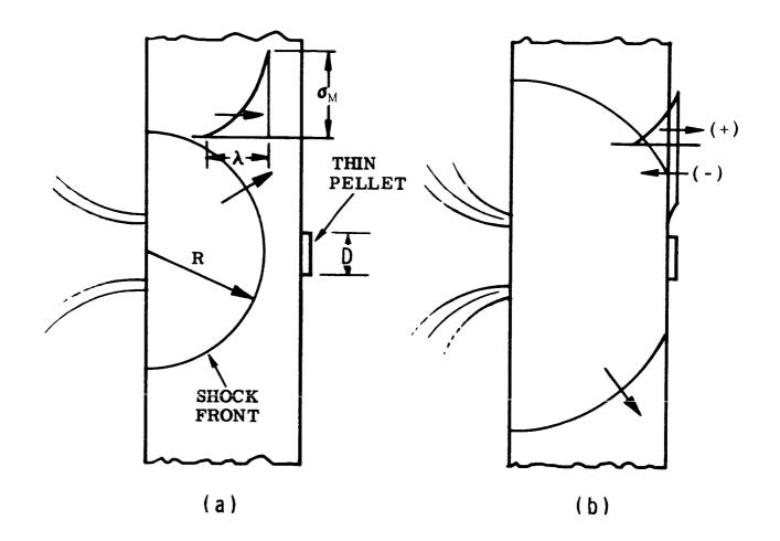
Figure 1 Fundamental Mechanism of the "Throw-Off-Pellet" Technique
