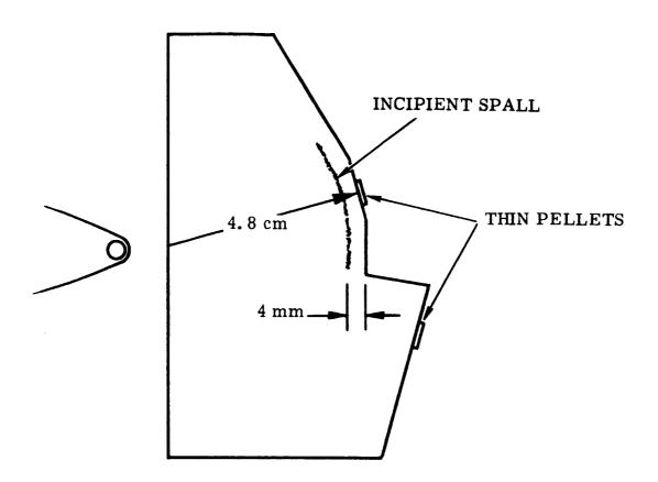
Figure 5 Special Target Used for Observing Incipient Spall
