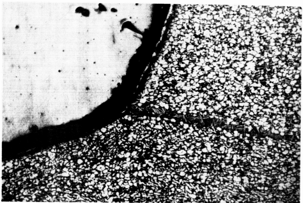
FIGURE 20 SURFACE AND BOND LINE CONTAMINATION - PACK #7
