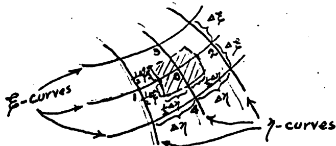
Fig. 4-1 Schematic Diagram of z - \eta Grid Points
