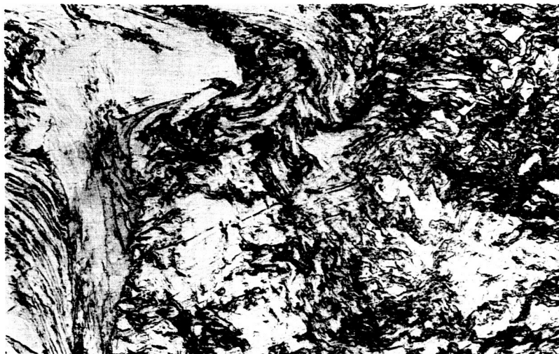
HARDNESS: DPH 278 ANNEALED 1 HOUR AT 2500°F (1371°C)
