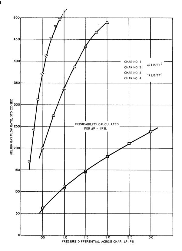
Figure 2. Permeation of Helium Gas Through Chars
