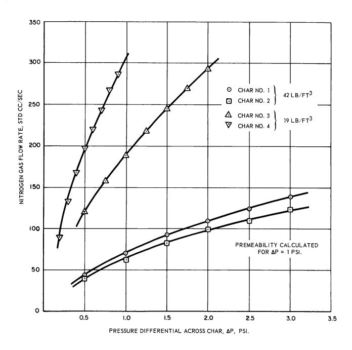
Figure 1. Permeation of Nitrogen Gas Through Chars
