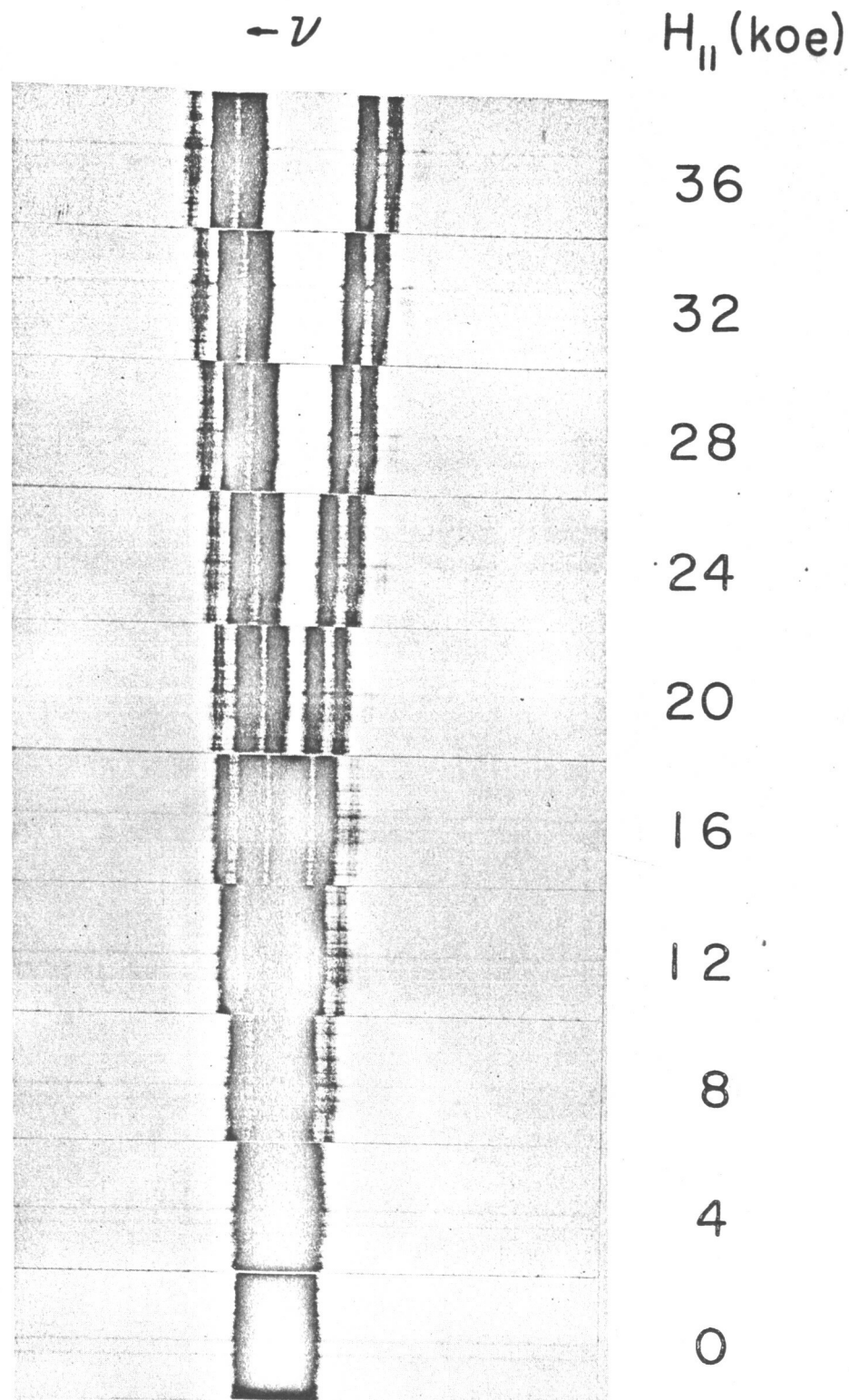
Figure 9. Parallel Zeeman splitting of I_1 ( \pi ) in \text{NdBr}_3 . Bath temperature is 1.5^\circ \text{K} . Region shown is centered at \lambda_{\text{vac}} = 4241 \text{ \AA} and is 5 \text{ \AA} ( 30 \text{ cm}^{-1} ) wide.
