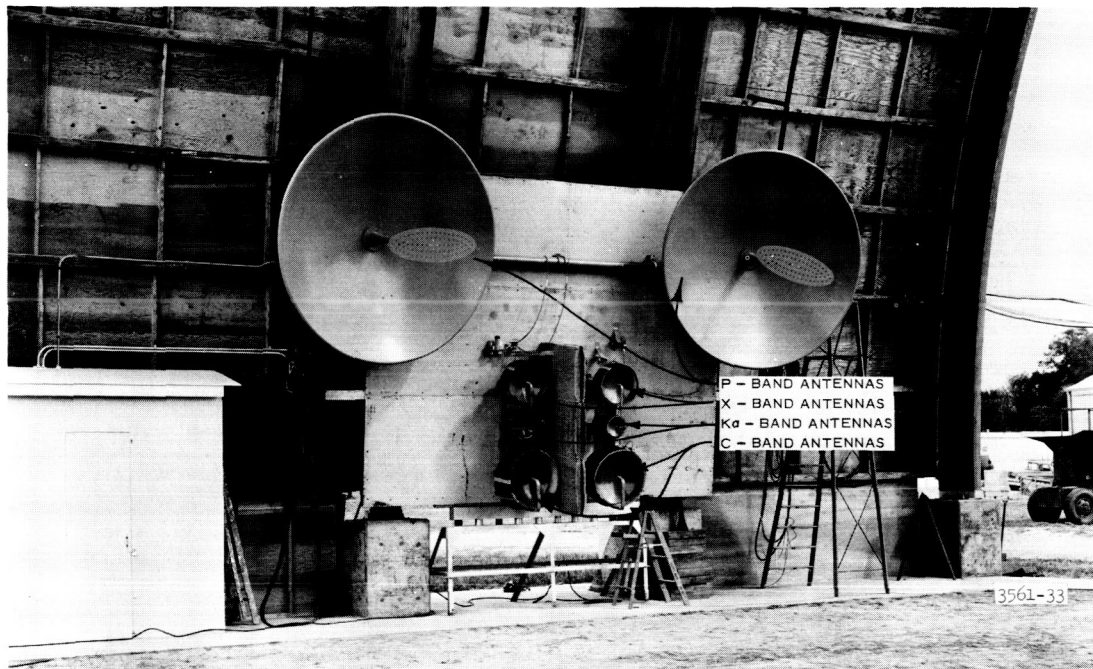
Fig. 2. Antenna carriage system
