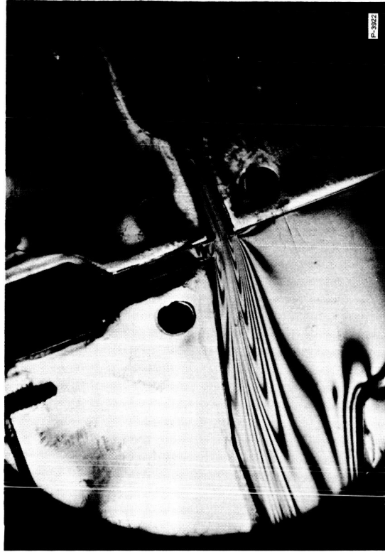
Figure 5-7 - Monostable Flip Flop, 30 Percent Supply Flow, Zero Control Flow, 25°C, Circularly Polarized Monochromatic Light
