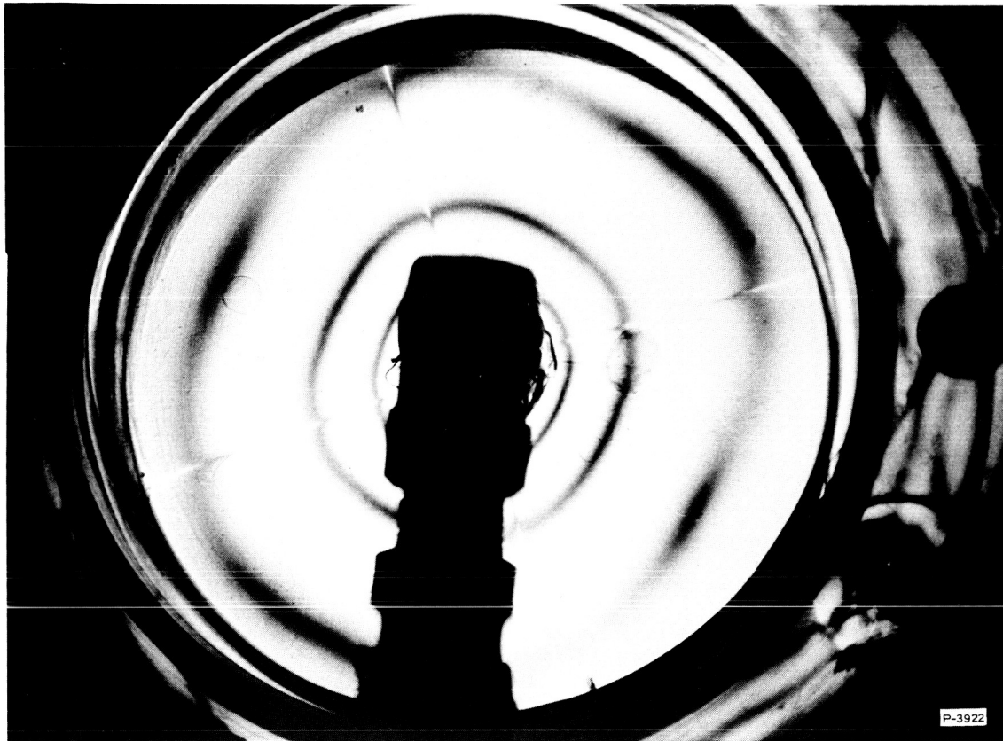
Figure 5-4 - Vortex Valve, 55 Percent Supply Flow, Zero Control Flow, 18.2°C, Circularly Polarized Monochromatic Light
