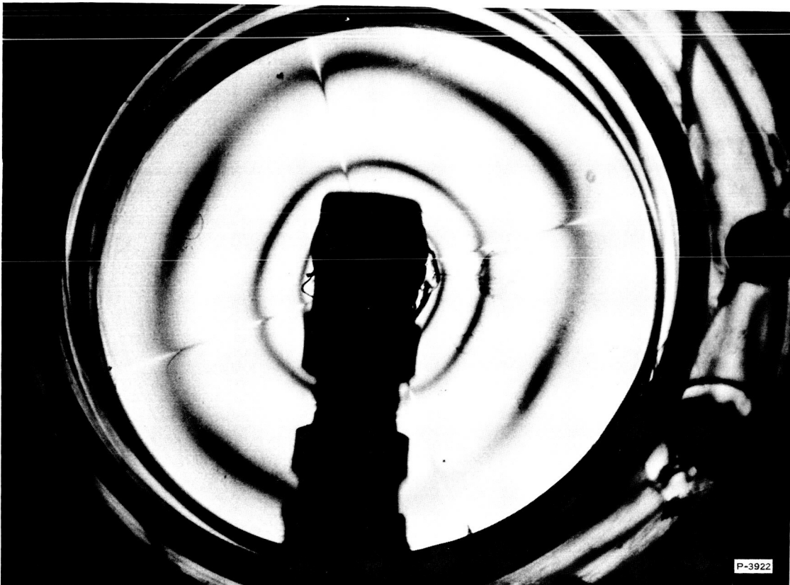
Figure B-1 - Vortex Valve, 50 Percent Supply Flow, Zero Control Flow, 18.2°C, Circularly Polarized Monochromatic Light
