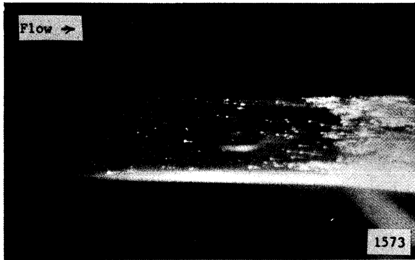
Fig. 2.--Typical photograph of air bubbles in 1/2" plexiglas venturi with water.
