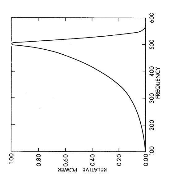
Fig. 2. Frequency response of the 525 Hz minus 500 Hz filter described in text.
