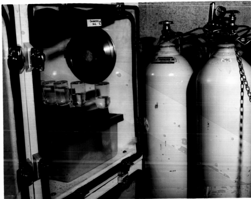
Figure 1. One of a battery of 4 chambers used for exposing mice to altered O_2 tensions at one atmosphere (normal) pressure.
