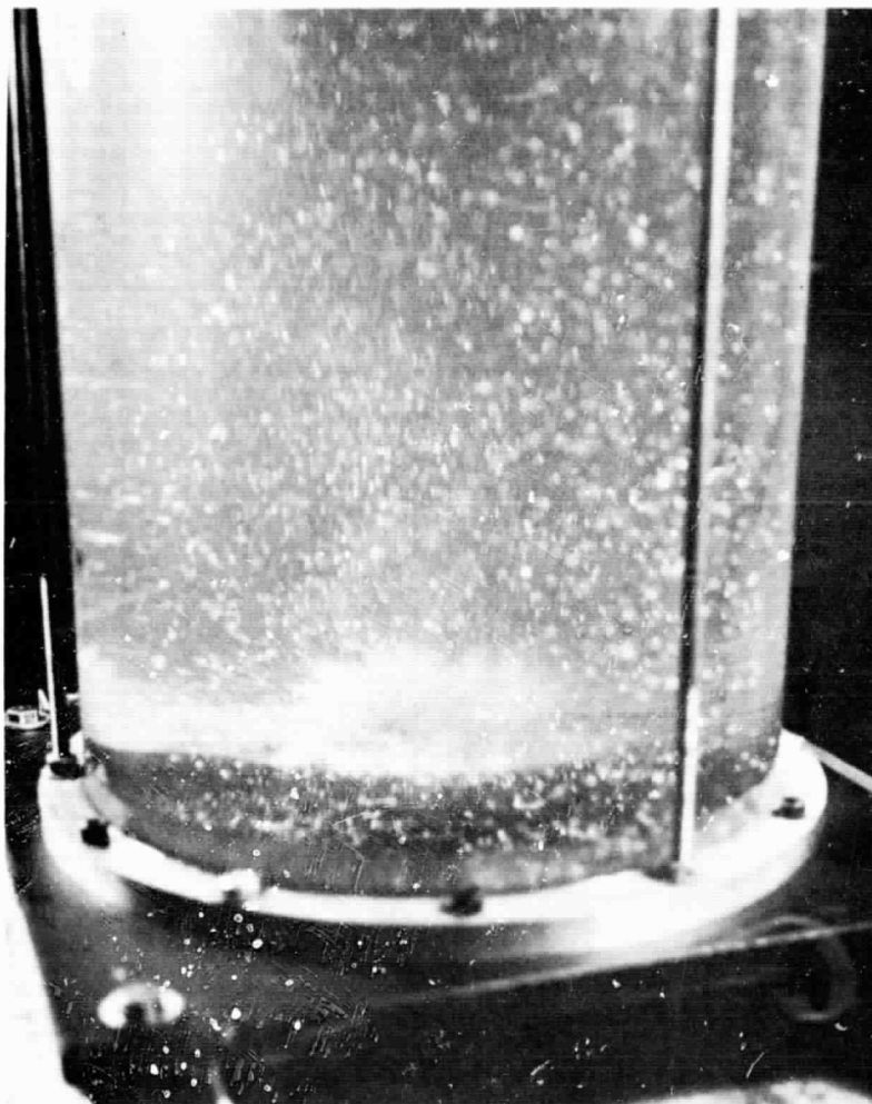
Figure 15. Large Bubble Cluster Forming By Small Gas Bubbles Sinking To Tank Bottom Under The Influence Of Longitudinal Excitation
