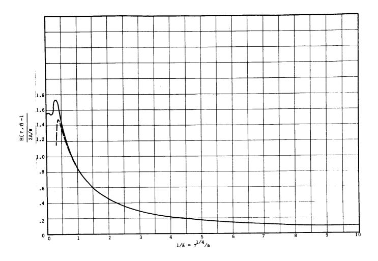
Fig. A-1 Time History of the Symmetry Point of a Disturbance in the form of a Square Wavelet
