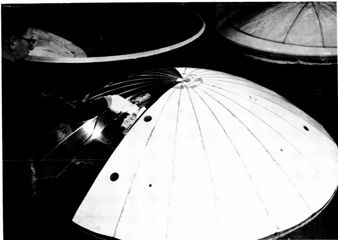
Figure 11. - Partially completed lay-up of gores on mold.
