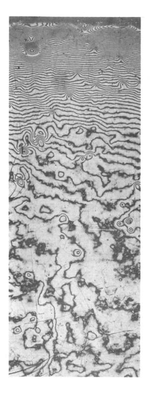
Figure IV-5. Interference Fringe Pattern from W9 after Heat Treatment, Showing Edge, 74x.
