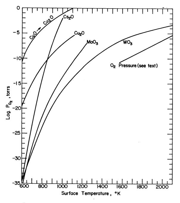
Figure V-34. Oxygen Pressure in Equilibrium with Various Metal Oxides as a Function of Temperature.
