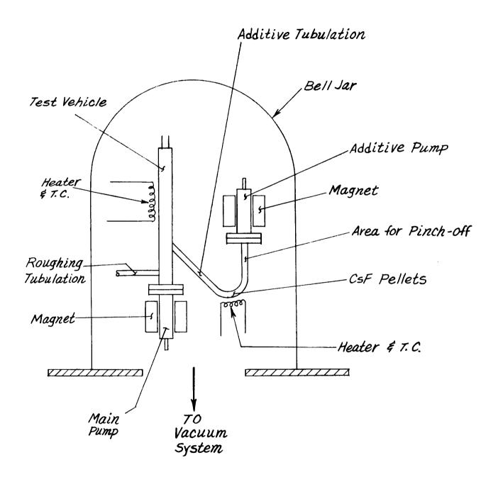
Figure V-7. Outgassing Set-up for Surface-Studies Device.
