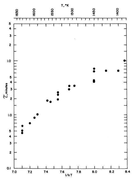
Figure V-17. Decay-Time Constant for CsF Coverage as a Function of Filament Temperature.
