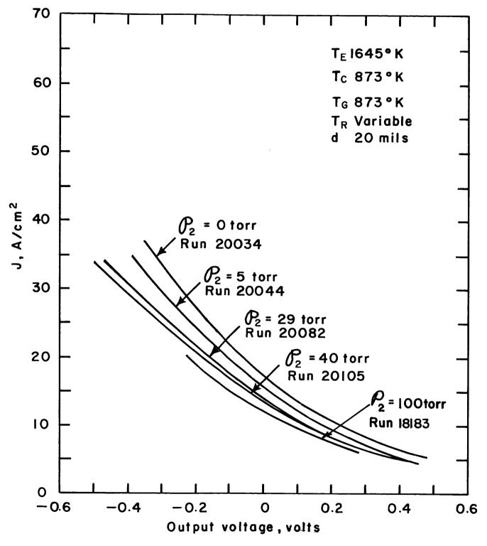
Figure VII-17. Variable-Reservoir-Temperature Envelopes at  $T_E = 1645^{\circ}K$  and d = 20 mils.
