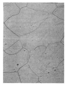
Figure IV-3. Emitter W9 after Heat Treatment, 310x.
