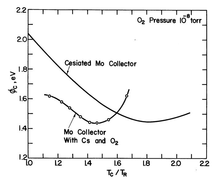
Figure V-38. Cesiated Collector Work Function Comparison With and Without Oxygen.
