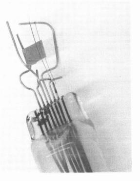
Figure V-30. Typical Glass-Tube Press with Electrodes.
