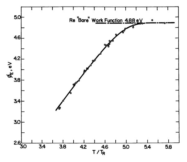
Figure VI-6. Work Function vs Surface-to-Reservoir Temperature Ratio Plot of Cesiated Work Function Measurements.
