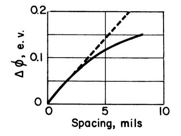
Figure VIII-3. Variation in Collector Work Function with Spacing.  $T_E = 1314^{\circ}K$ ,  $T_C = 609^{\circ}K$ ,  $T_R = 543^{\circ}K$
