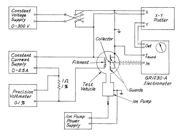
Figure V-8. Circuit Diagram for Emission Measurements.
