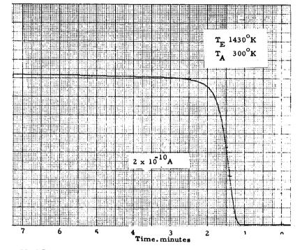
Figure V-12. Emission Current Transient for Step Change in Filament Heating Current, No CsF.
