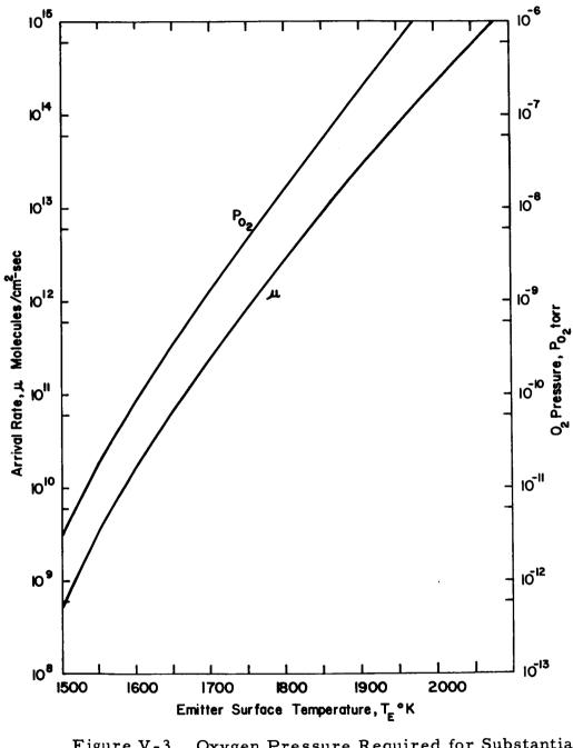
Figure V-3. Oxygen Pressure Required for Substantial Coverage as a Function of Surface Temperature.
