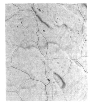
Figure IV-4. Emitter W10 after Heat Treatment, 310x.
