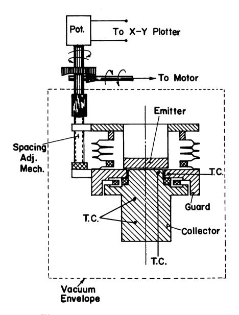
Figure VIII-2. Schematic of the Cesium Diode.
