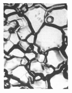
Figure IV-10. Re31 after Heat Treatment, 310x.
