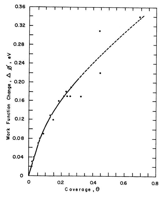
Figure V-18. Surface Work Function Change Produced by CsF Coverage.
