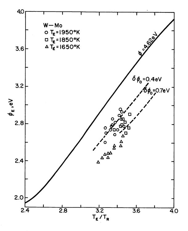
Figure V-1. Experimental and Theoretical Cesiated-Surface Work Functions with Electronegative Additive.
