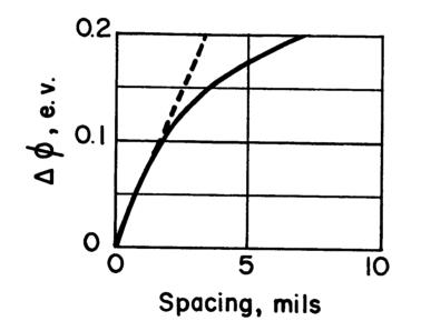
Figure VIII-6. Variation in Collector Work Function with Spacing.  $T_{E} = 1308^{\circ}K$ ,  $T_{C} = 621^{\circ}K$ ,  $T_{R} = 593^{\circ}K$ .
