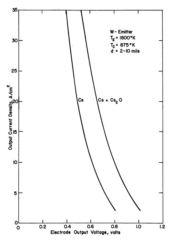
Figure V-36. Performance Envelope with  $Cs_2O$  and Cesium.
