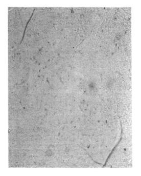
Figure IV -1. Emitter W9 after Electropolishing, 310x.
