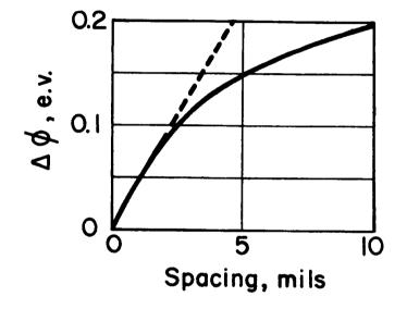
Figure VIII-5. Variation in Collector Work Function with Spacing.  $T_{E} = 1298^{\circ}K$ ,  $T_{C} = 618^{\circ}K$ ,  $T_{R} = 572^{\circ}K$ .
