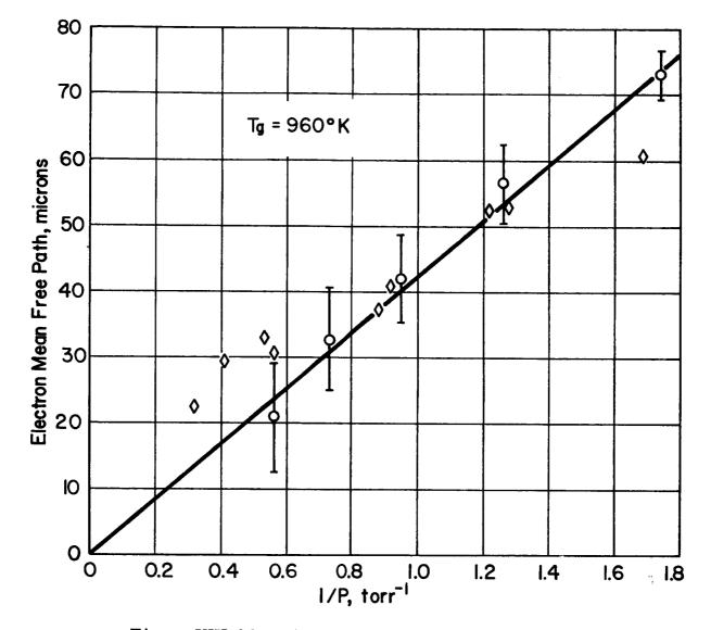
Figure VIII-10. Electron Mean Free Path in Cesium Vapor.
