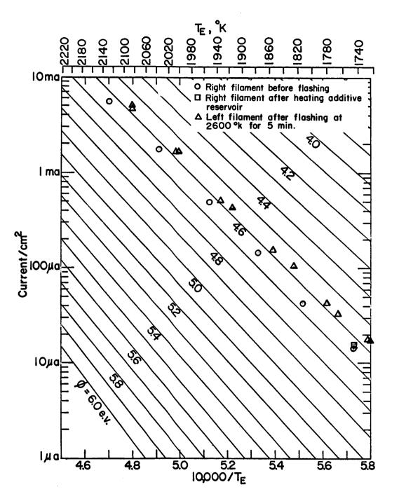
Figure V-10. Right Filament Work Function with Liquid Nitrogen Cooling.
