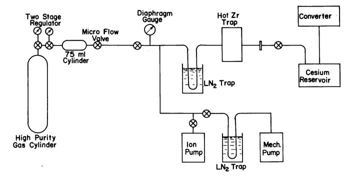
Figure VII-2. Schematic of the Standard Gas Injection System.
