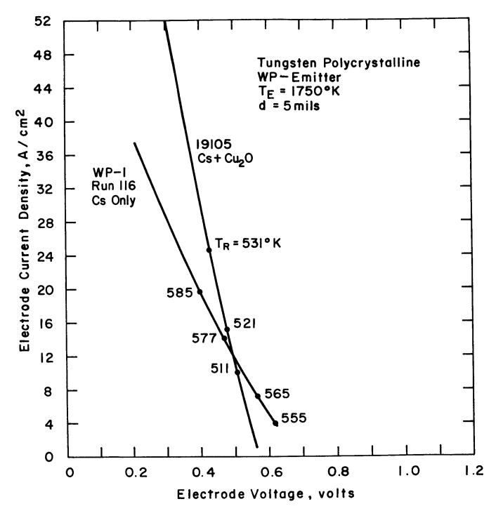
Figure V-45. Performance Envelope Comparison Cs Only and Cs plus Cu<sub>2</sub>O, T<sub>f</sub> 1750 °K.
