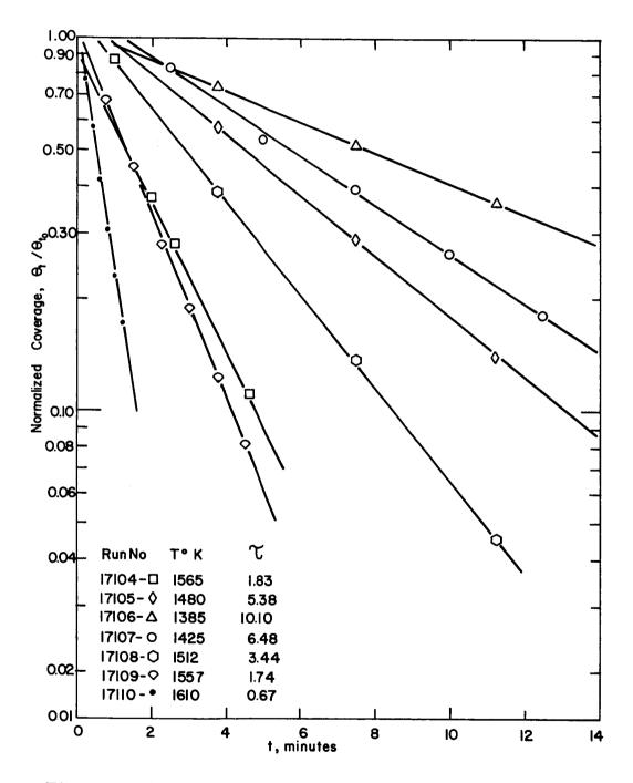
Figure V-16. Characteristic Decay of CsF Coverage for Several Filament Temperatures.
