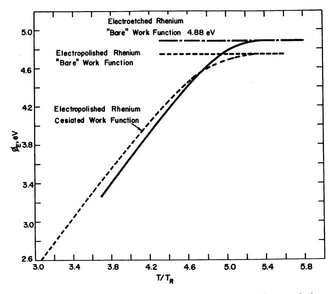
Figure VI-7. Comparison of the Work Functions of Electroetched and Electropolished Rhenium.
