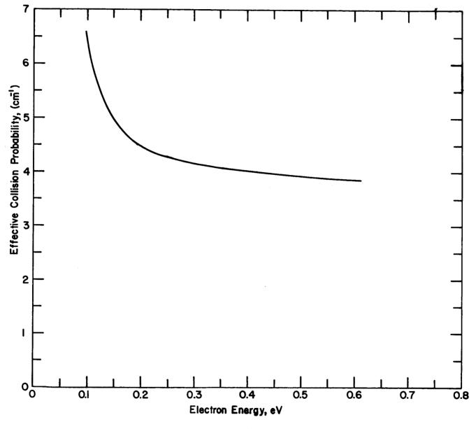
Figure VII-10. Effective Collision Probability of Electrons with Argon.
