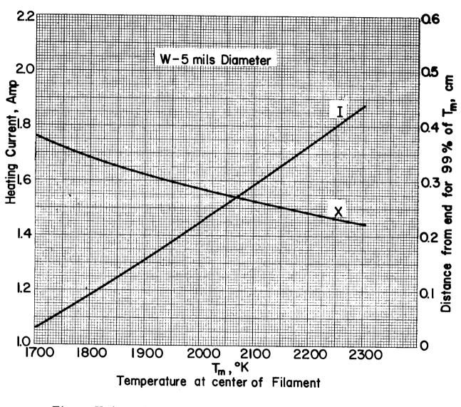
Figure V-6. Filament Temperature as a Function of Heating Current and Influence of End Connections on Temperature Uniformity.
