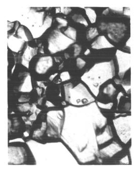
Figure IV-8. Emitter Re31 after Electroetching, 310x.
