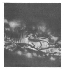
Figure V-33A. Micro-Photograph of Tungsten Filament Eroded in a Glass Tube.
