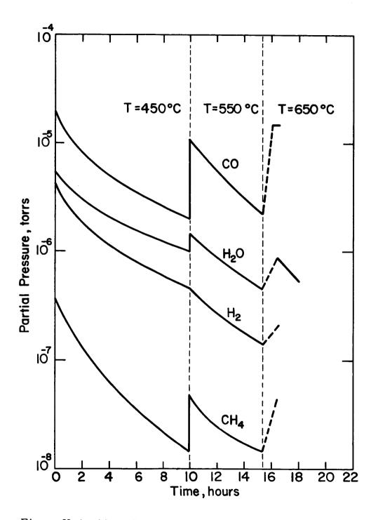
Figure V-4. Mass Spectrometer Analysis of CsF Outgassing.
