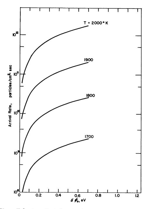
Figure V-2. Bare-Work-Function Shift Produced by Oxygen Additive.
