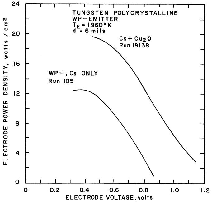
Figure V-46. Power-Density Comparison of Cs Only and Cs plus Cu<sub>2</sub>O, T<sub>r</sub> 1960 °K.
