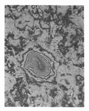
Figure IV-7. Interference Fringe Pattern from W10, Showing Polishing Defect, 152x.
