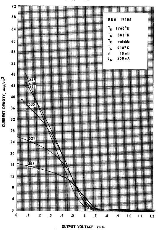
Figure V-40. J-V Family with Cu<sub>2</sub>O Additive,  $T_{E}$  1760 °K.
