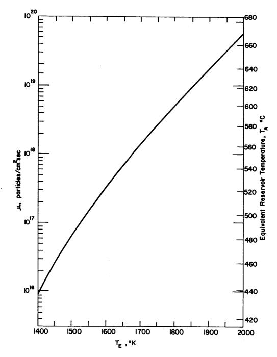
Figure V-19. CsF Arrival Rate Required to Maintain Half a Monolayer Coverage at a given Surface Temperature
