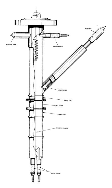
Figure V-5. Drawing of Surface Studies Device
