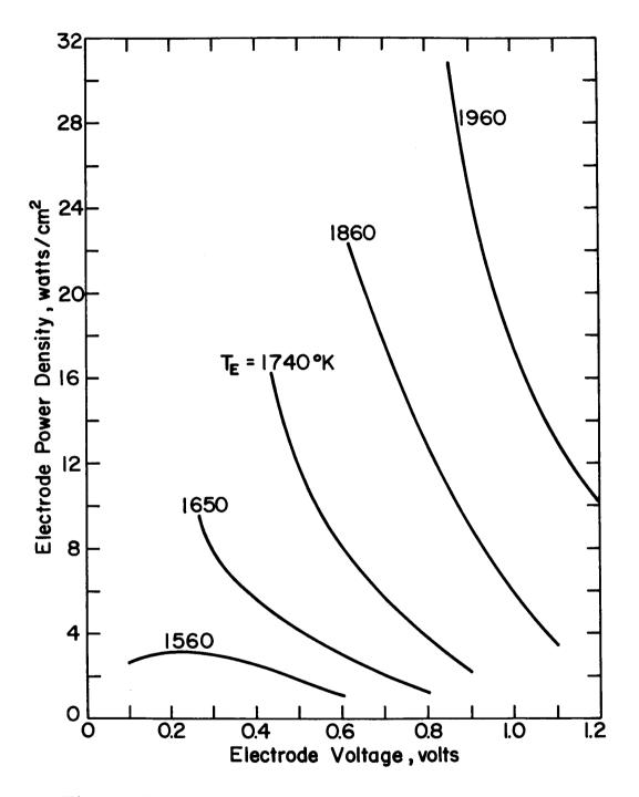
Figure VI-14. Fully Optimized Electrode Power Output Map.
