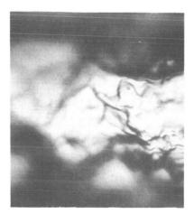
Figure V-33B. Micro-Photograph of Tungsten Filament Eroded in a Glass Tube.
