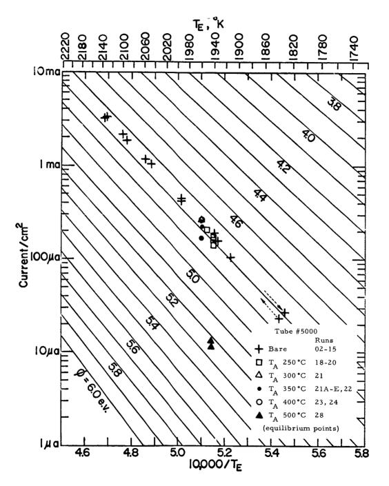
Figure V-20. Saturation Current vs Reciprocal Emitter Temperature for Bare Surface.
