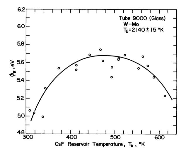
Figure V-32. Work Function Change Produced in CsF Glass Tube.
