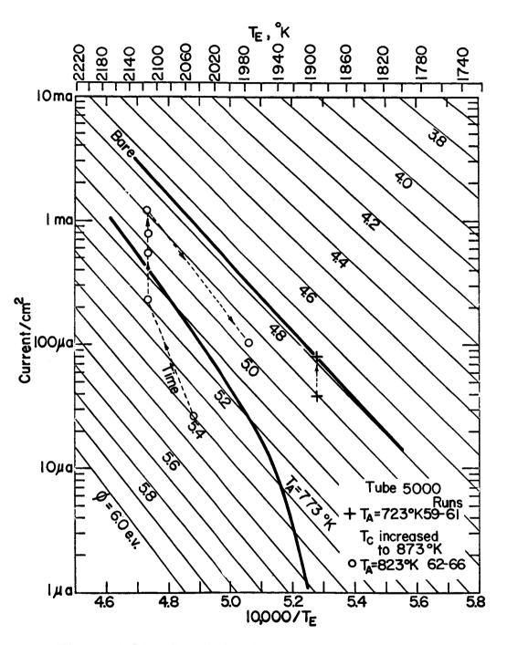
Figure V-24. CsF-Only Work Functions in Converter 5000.
