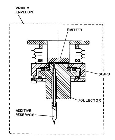
Figure V-37. Schematic of Parametric Converter Showing Additive Reservoir.
