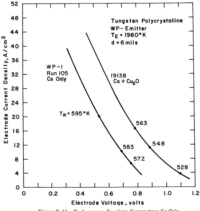
Figure V-43. Performance Envelope Comparison Cs Only and Cs plus Cu<sub>2</sub>O, T<sub>E</sub> 1960°K.
