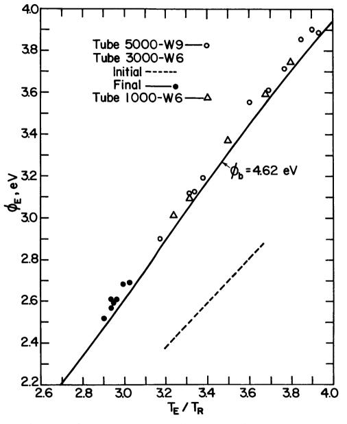
Figure V-29. Comparison of Cesiated  $\phi$  for Various CsF Converters.
