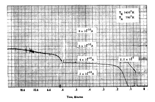
Figure V-13. Emission Current Transient for Step Change in Filament Heating Current, Constant CsF Arrival Rate.
