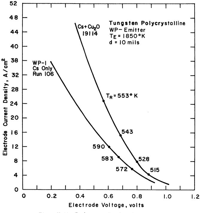
Figure V-44. Performance Envelope Comparison Cs Only and Cs plus  $Cu_2O$ ,  $T_E$  1850 °K.
