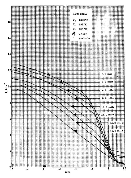
Figure VII-4. Typical Variable-Spacing Electrical Output Characteristic.
