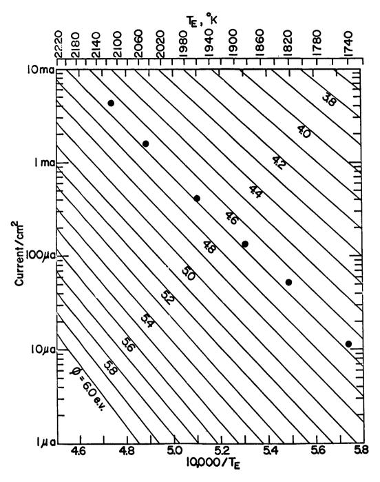
Figure V-9. Left Filament Work Function, No Liquid Nitrogen Cooling.
