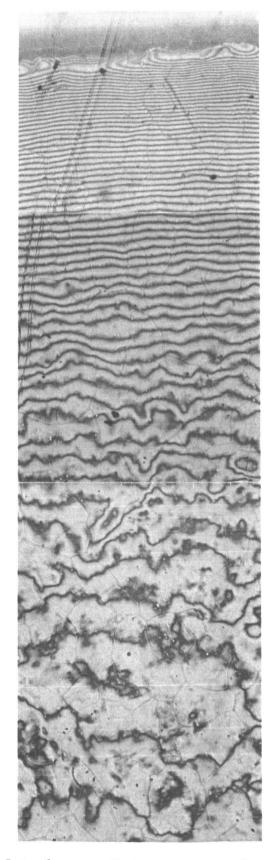
Figure IV-6. Interference Fringe Pattern from W10 after Heat Treatment, Showing Edge, 152x.
