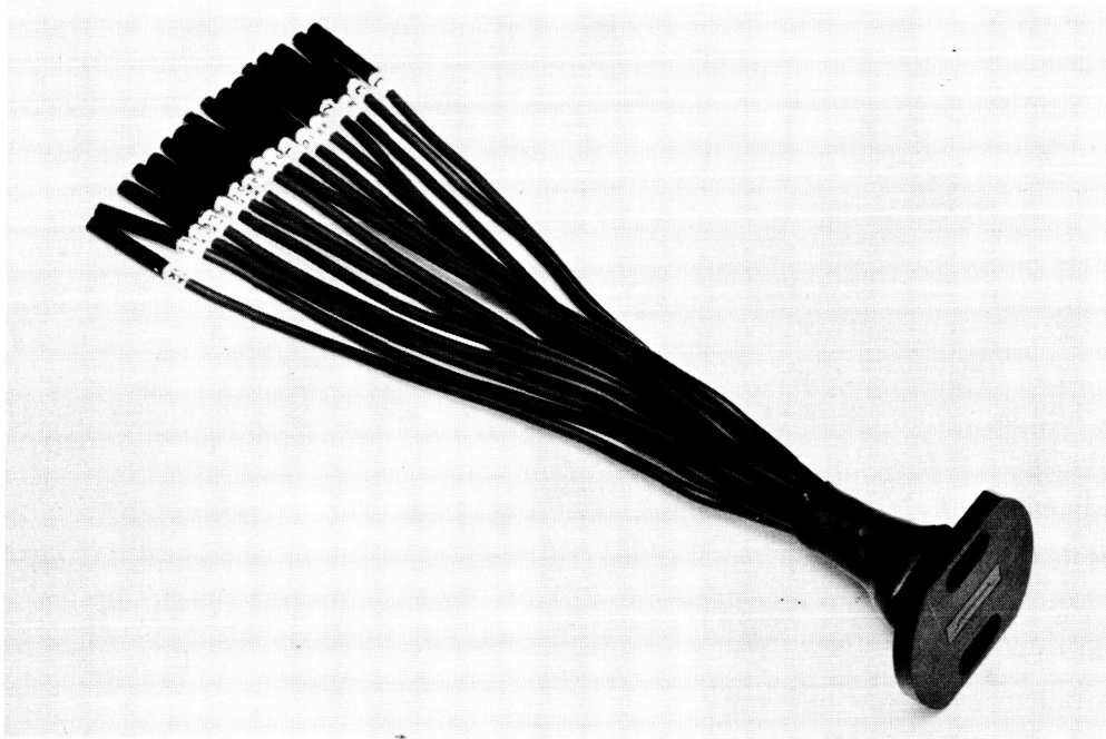
FIGURE 38. FIBER OPTICS OF EXISTING SPECTROMETER DETECTOR SYSTEM
