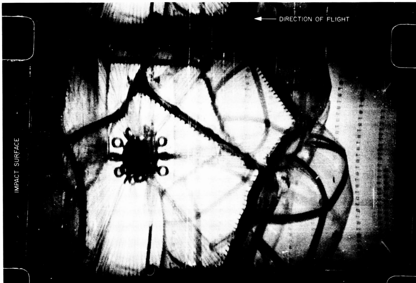
Fig. 17. Impact limiter fully deflected, 100-ft/sec
