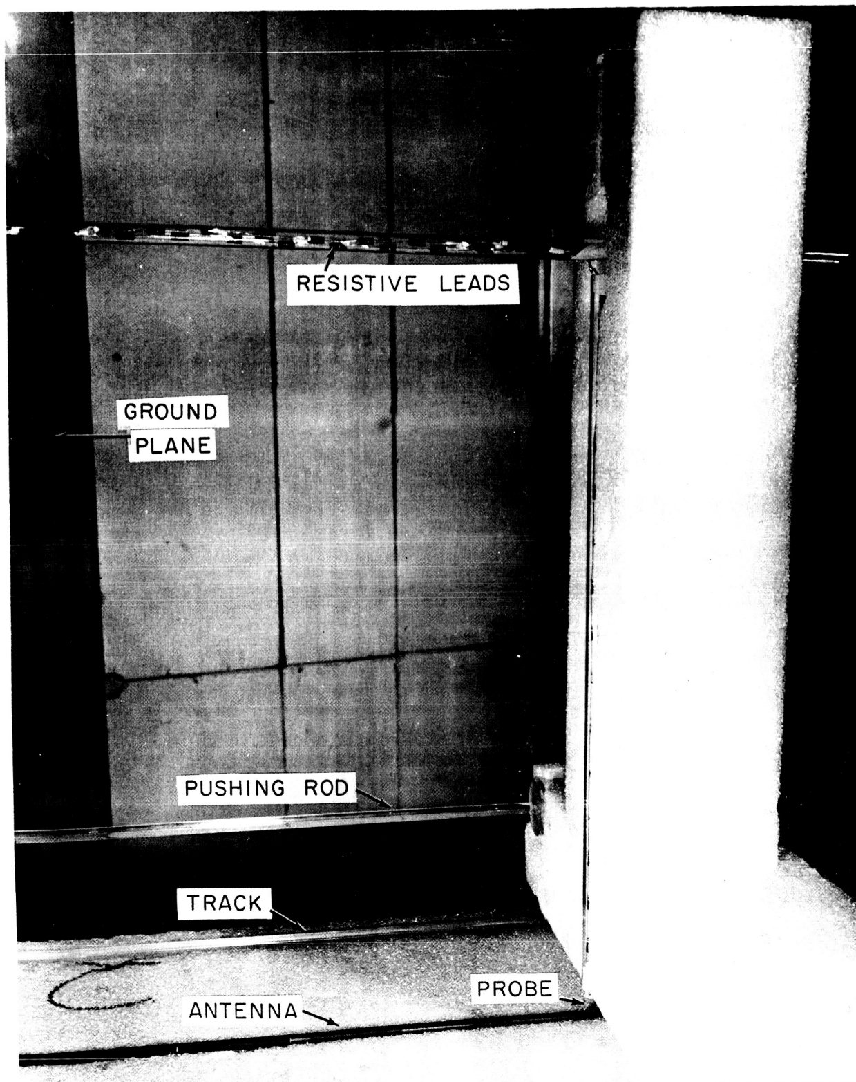
FIG. 5 THE EXTERNAL PROBE AND ITS SUPPORTING STRUCTURE
