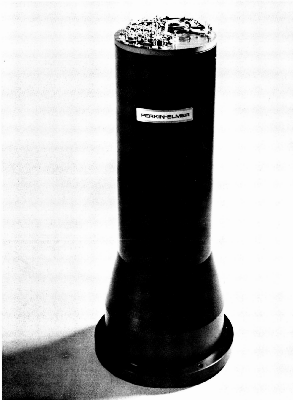
Figure 3-10. Photograph of Complete Coarse Acquisition Detector Assembly
