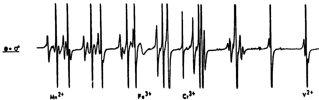
Fig. 2.3. ESR spectra of V^{2+} , Cr^{3+} , Mn^{2+} and Fe^{3+} in a single crystal of CaO at \theta = H \wedge [100] = 0 and T = 300^\circ K
