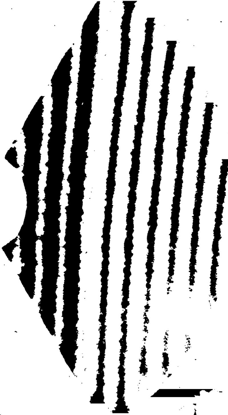
Interferogram of mirror segment taken with scatterplate interferometer. Linearity and spacing of fringes are measured to determine quality of segment figure. Measurements show that the rms figure error is less than  $1/20\lambda$ .
