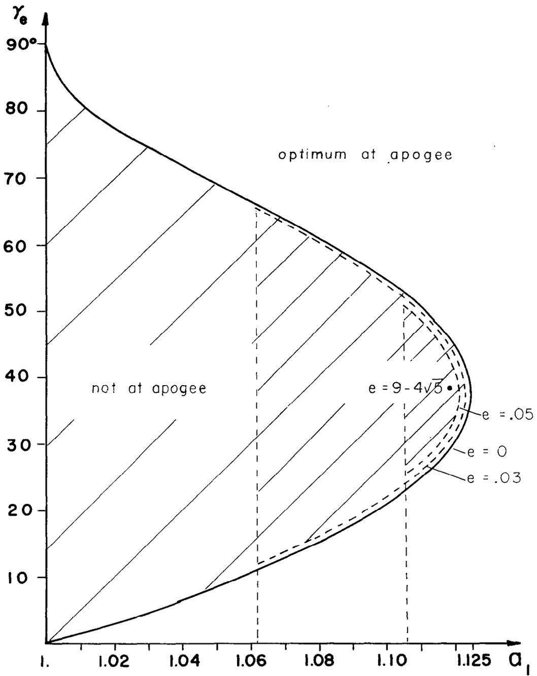
FIG. 9. CONDITIONS FOR OPTIMUM DISORBIT AT APOGEE
