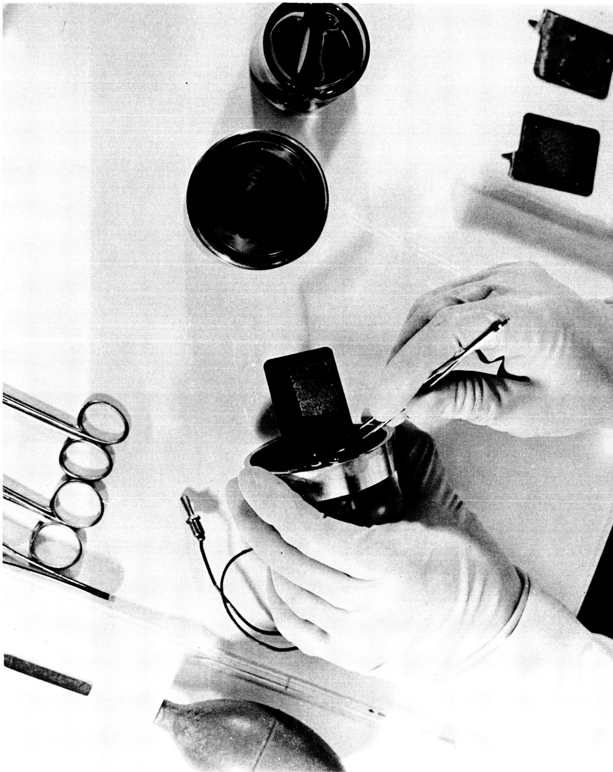
FIGURE 1. ASSEMBLY OF STAINLESS STEEL-CASED CELL FOR SILVER ELECTRODE STUDIES
