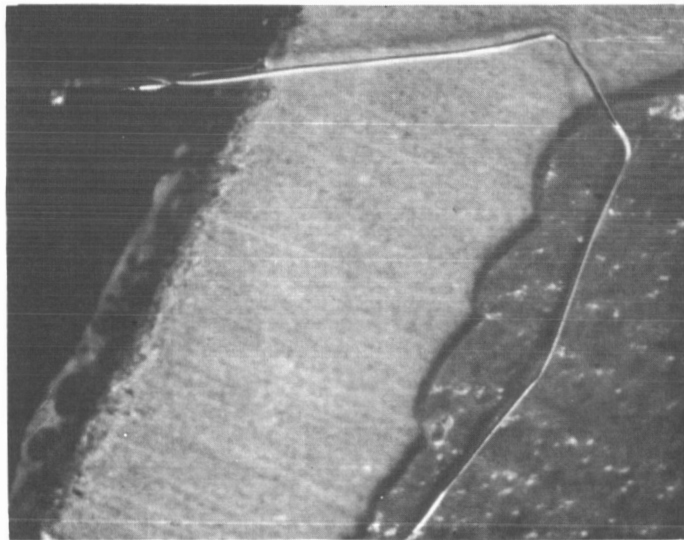
Figure 2-10 Optical Confirmation of Figure 2-9 (Extraneous Gold Wire Was Located Within Case and Between Lid and Case Body)
