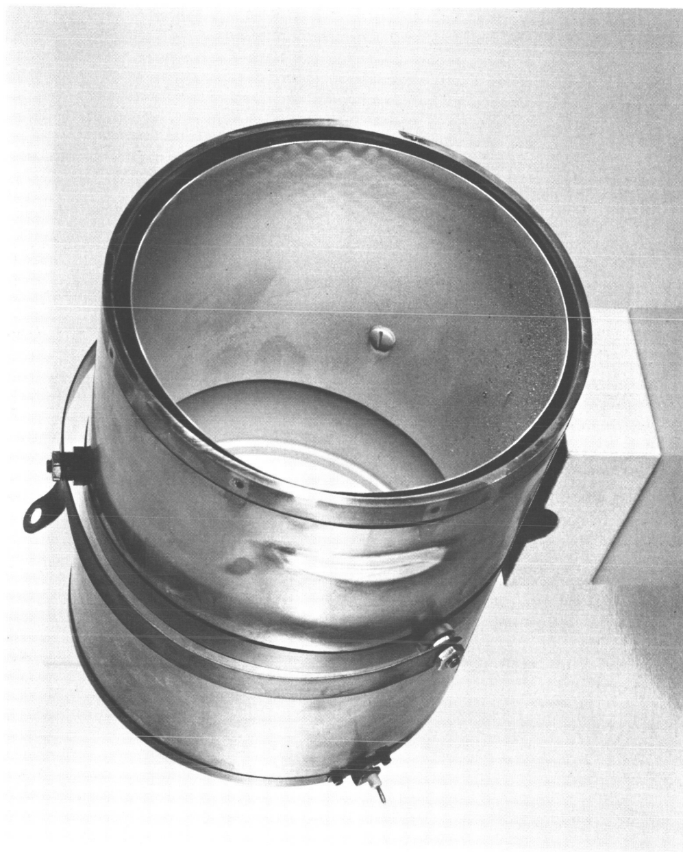
Figure 60. DG-2 Engine Shell After 3149-Hour Test
