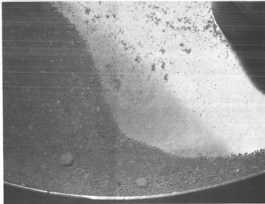
FIG. 20. Spherical shaped aggregates produced in the collecting pan by air grinding.
