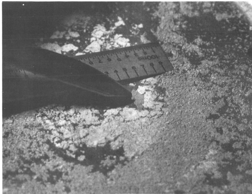
FIG. 18. Self supporting flake of powder resulting from compression of free powder on the pan after vacuum grinding.
